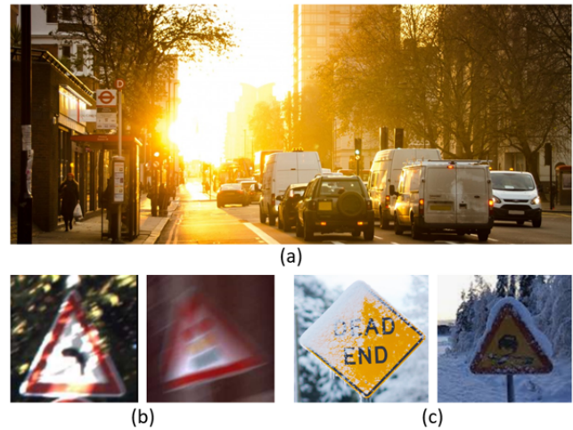
Fig. 23. Challenges in traffic sign detection and traffic light detection: (a) Illumination changes. Image from pxhere (free of copyrights). (b) Motion blur. Image from GTSRB Dataset [81]. (c) Detection under bad weather. Image from Flickr and Max Pixel (free of copyrights).
